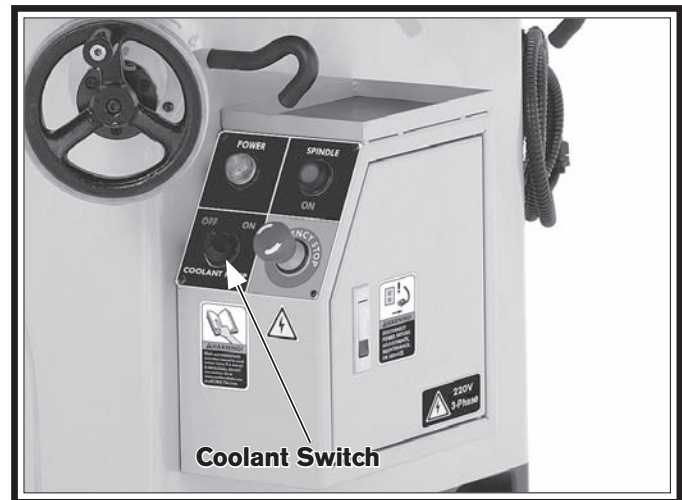
Figure 3. SB1029 control panel.
